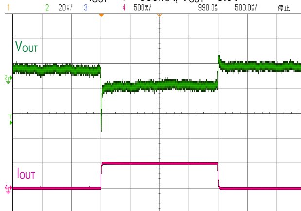
Load Transient Response I_{OUT} = 1 \sim 500\text{mA} , V_{OUT} = 3.3\text{V}
